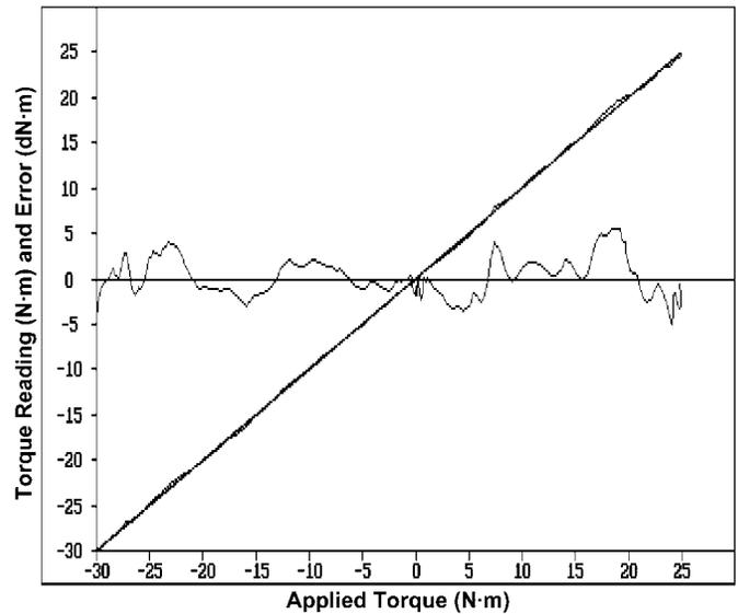
**Figure 15:** Calibration of stall torque measurement with electronic torque wrench
