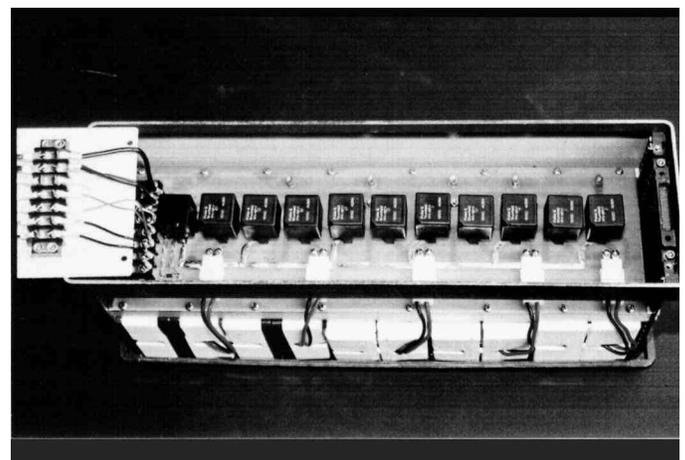
**Figure 9:** Interior of battery box with 5 amp-hour batteries
