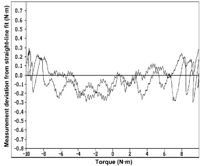
**Figure 18:** Torque measurement error band
