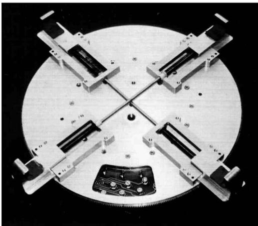
**Figure 8:** "Skate key" synchronous clamp assembly
