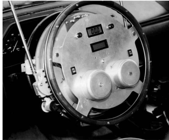
Figure 1: Machine installed in a test vehicle
