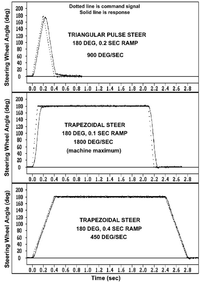
**Figure 13:** Response to commanded ramps in pulse and trapezoidal steer
