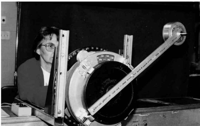
**Figure 16:** Pendulum test for torque measurement
