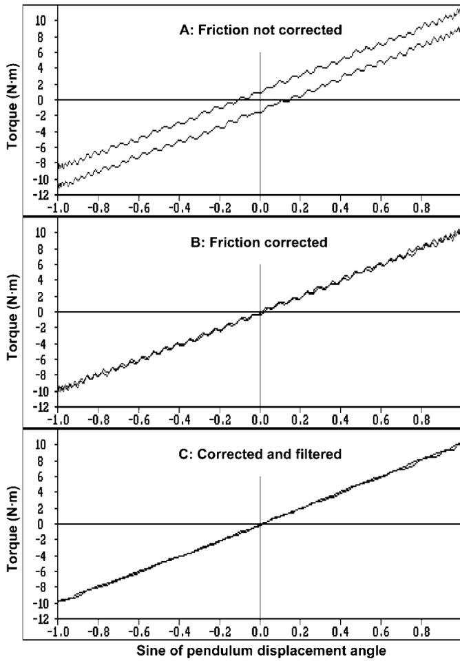
**Figure 17:** Torque measurement in pendulum test
