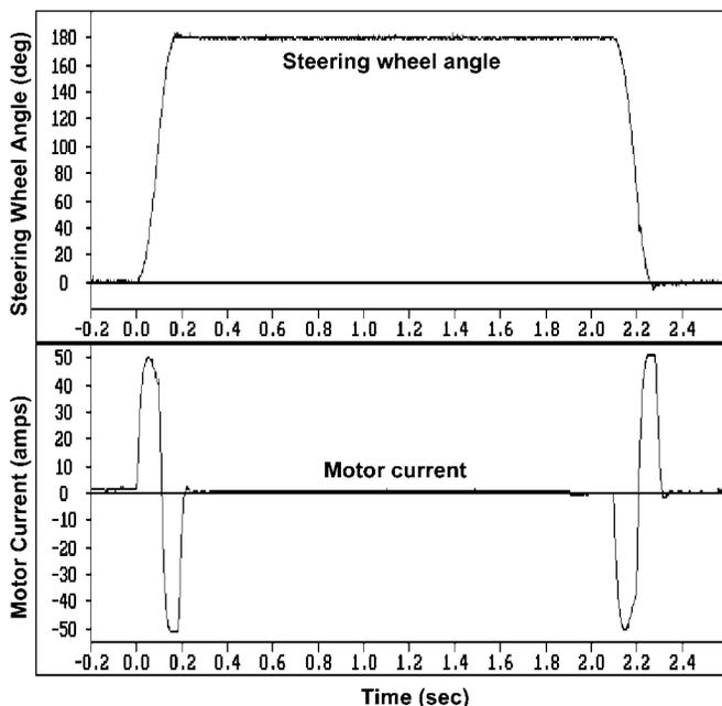
Figure 11: Motor current during 180 deg, 0.1 sec steer ramps
