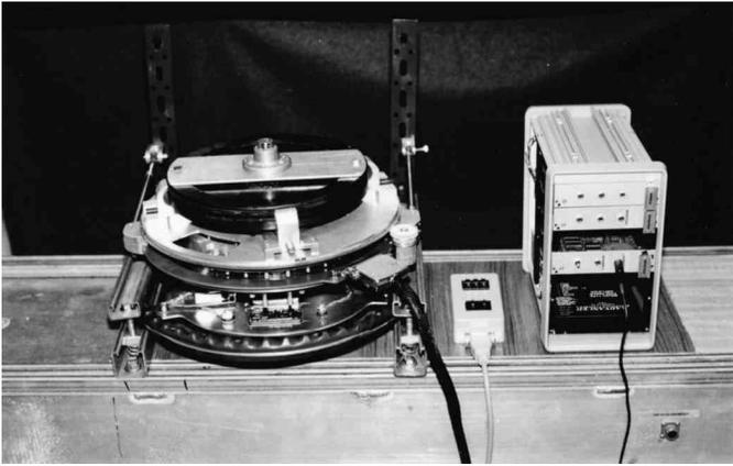
**Figure 12:** Test bench setup with barbell weight to simulate a vehicle steering system
