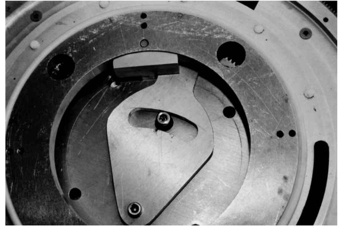
**Figure 7:** Removable  $\pm 180$  degree safety stop
