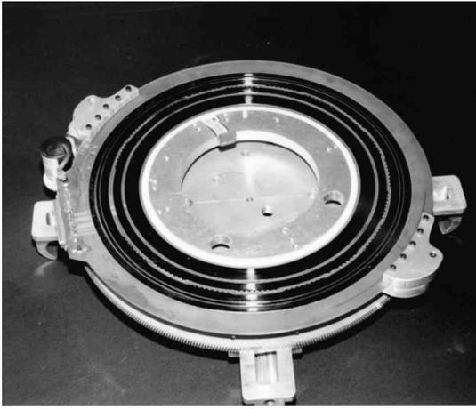
**Figure 6:** Grounding disk/slip ring assembly
