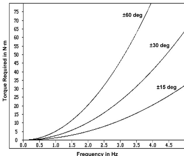
**Figure 10:** Torque required in frequency response testing
